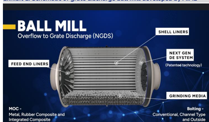
Exhibit 1: Schematic of grate discharge ball mill developed by AIAE
